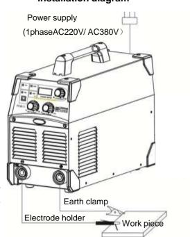
If distance of work piece and machine is too far (50-100m), and the cables (torch cable and earth cable) are too long, please choose cable of bigger section to minimize the reduction of the voltage.
